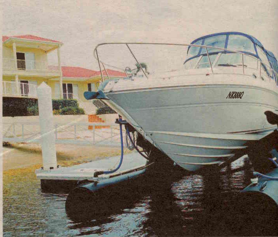
AIRBERTH uses the buoyancy of air to raise the boat out of the water.
