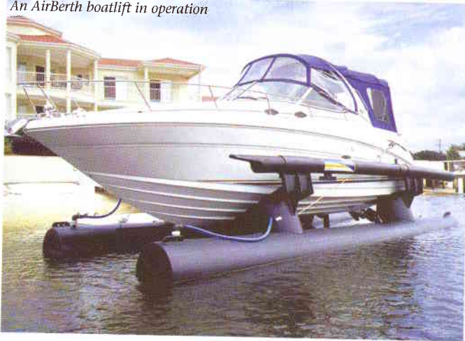
An AirBerth boatlift in operation
