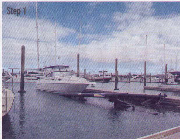
Drive the boat onto the submerged AirBerth and secure the positioning ropes to the boat.
