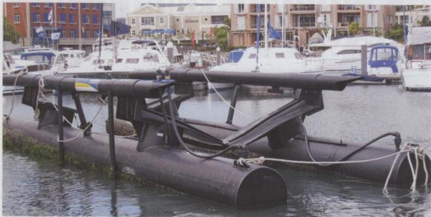
The Air Berth rises above the water as air is supplied to the main buoyancy chambers and water is pumped out through the tailpipes.
