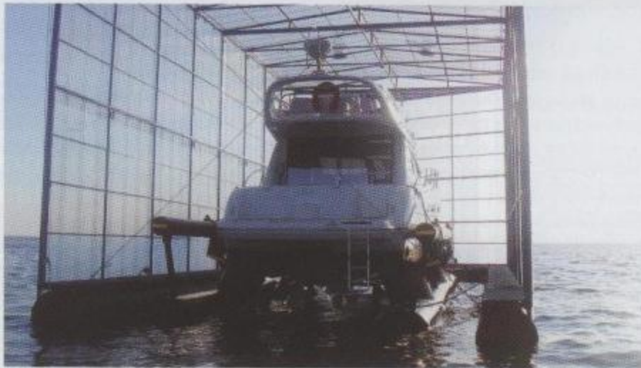
The Air Berth rises above the water as air is supplied to the main buoyancy chambers and water is pumped out through the tailpipes.
