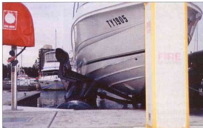
Fully clear of the water, the Mustang's gleaming, un-treated hull receives a wash-down from spray rails on both sides of the AirBerth - hose is then used to flush both Volvo Penta engines...
