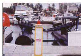
Front view of AirBerth - Graeme attaches air hoses, run by twin jacuzzi pumps, which plug into berth's shore-power...
