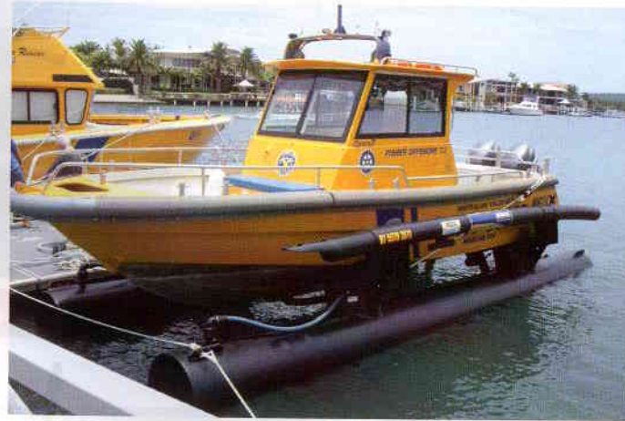
The boat lift keeps the hull well out to the water
