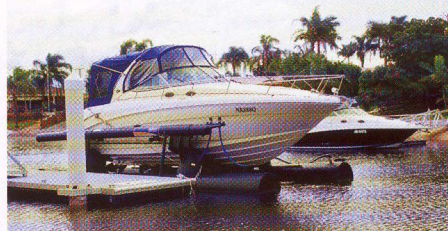
Semi-profile view of the AirBerth lifted boat. The submersible unit is barely wider than the boat it lifts
