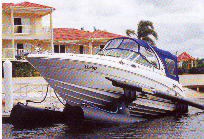
Semi-profile view of the AirBerth lifted boat. The submersible unit is barely wider than the boat it lifts
